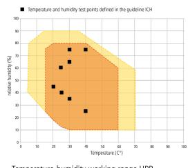
Temperature-humidity working range HPP • HPP110 - HPP1060 without light/ • HPP1400 & HPP2200 Standard units are safety-approved and bear the test marks
