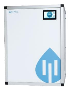
The ready-for-connection pure water system PROTEUS has been developed to economically produce high quality pure water and pump it, as required, to complete laboratory storeys and doctor's offices, where space is scarce. Pre-treatment, reverse osmosis, optional EDI purification steps, a pure water tank and a booster pump are compactly combined and mounted in a compact cabinet.
